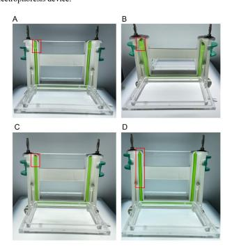
Note: When loading plastic boards, the low edge should face inward. If only single prefabricated gel electrophoresis is performed, please insert a baffle on the other side to prevent leakage of electrophoresis solution; Taking the raised sealing strip of the electrophoresis instrument as an example, if there is no raised surface, ignore this step.
